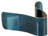
Ball Tension Spring (10) keeps a constant light tension on the Handle (3). The Ball Tension Spring can be removed by rotating the Handle all the way to the tight position, compress the spring together and pull the spring out. Re-installation is done in reverse.
